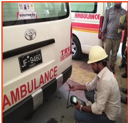
Vehicle Emission Monitoring
